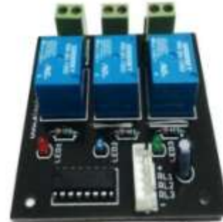
Fig. 14 Relay module with ULN2003 IC
